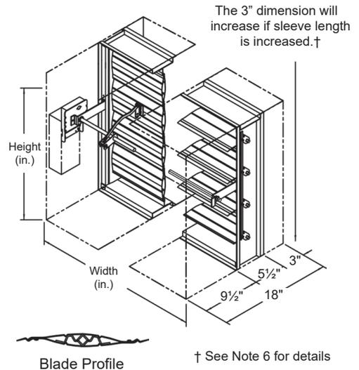
When using a true 6" high damper, width is limited to 16". If damper is ordered as 6" high and width is less than 16", an 8" high damper with 2" short-height transition will be supplied.
